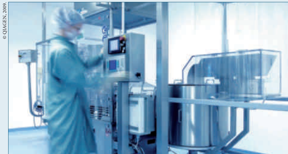
Biological production at QIAGEN: The machine fills enzymes produced by QIAGEN for the subsequent packaging in kits ready for use.
